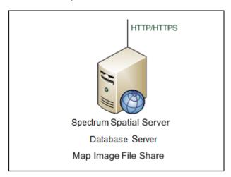
To scale Spectrum Spatial from one to three servers, each server leverages a single shared database server and image server to maximize efficiency and to avoid situations where an image or database resource is unavailable to one of the Spectrum Spatial servers. The file image server stores all images between multiple versions of Spectrum Spatial. All instances of Spectrum Spatial store images in a single location
