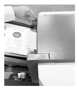
**NOTE**: Return this lever to its normal position when the feeder is used for automatic operation.
