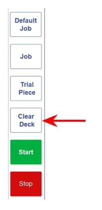
4. Tap the **Clear Deck** button to clear the paper path of any remaining material.
