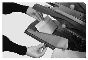
3. Aerate and fan the stack of envelopes so the individual envelopes are not stuck together.
