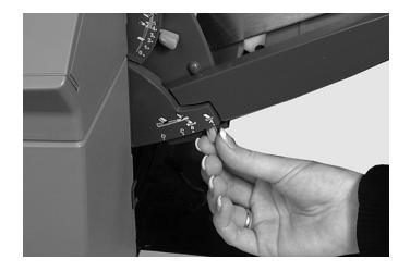
5. Set the blue separator shield lever to the letter required.
