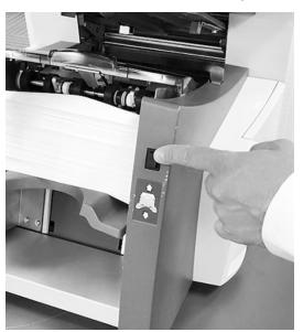
2. Use the side guide adjustment knob to adjust the side guides to the width of the envelopes. Once the guides are touching both sides of the envelope, turn the adjustment knob 1/4-turn in the opposite direction. This sets the correct clearance between the guides and the envelope.
