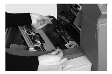
3. Remove the jammed material. If necessary, *use the manual advance knob* to move the material backwards.
