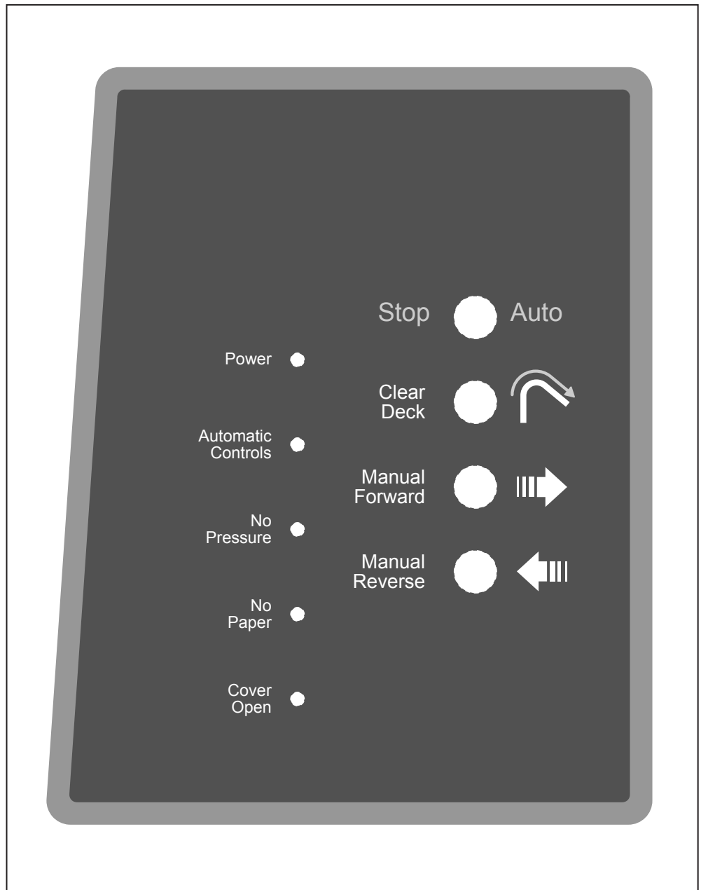
F734/F735 High Capacity Feeder Control Panel
