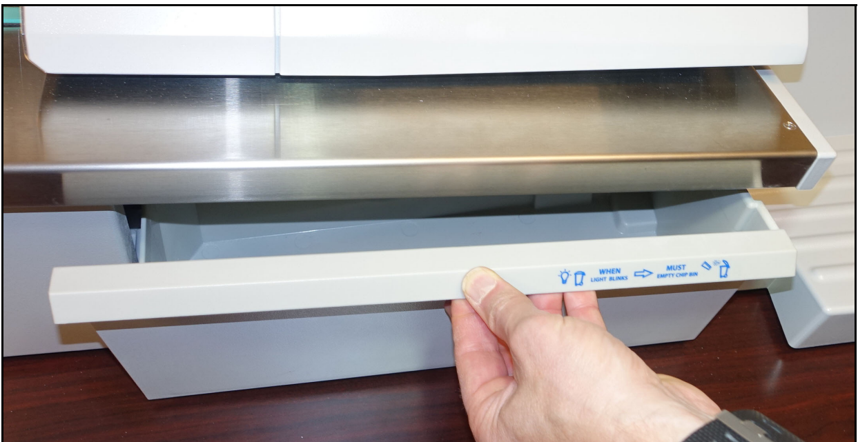
Figure 2-10: Bin tray removal interlock triggering
