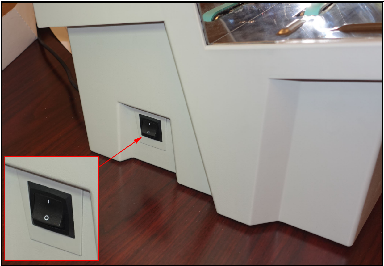
Figure 4-5: AC power switch
