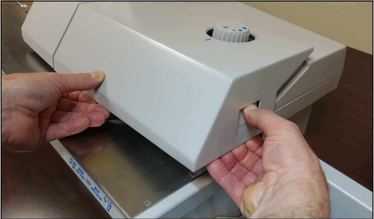
Figure 2-9: Top cover removal interlock triggering
