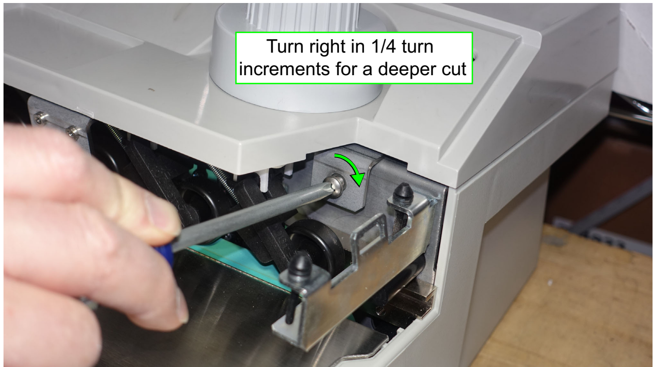
Figure 4-18: Adjusting the cutter depth
