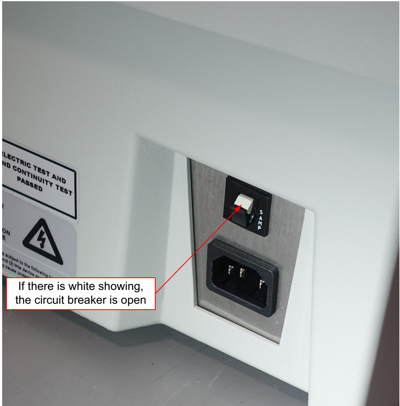
Figure 4-19: Open circuit breaker
