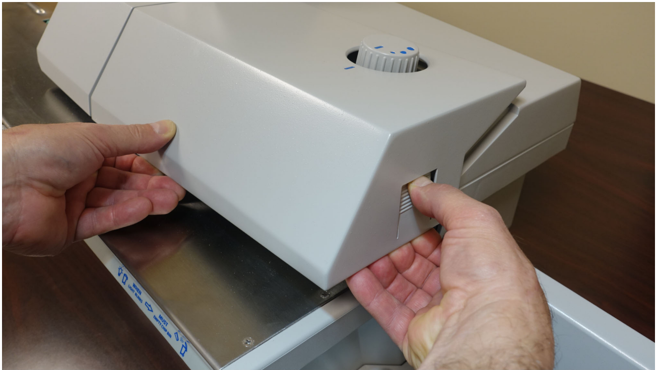
Figure 2-7: Top cover removal interlock triggering
