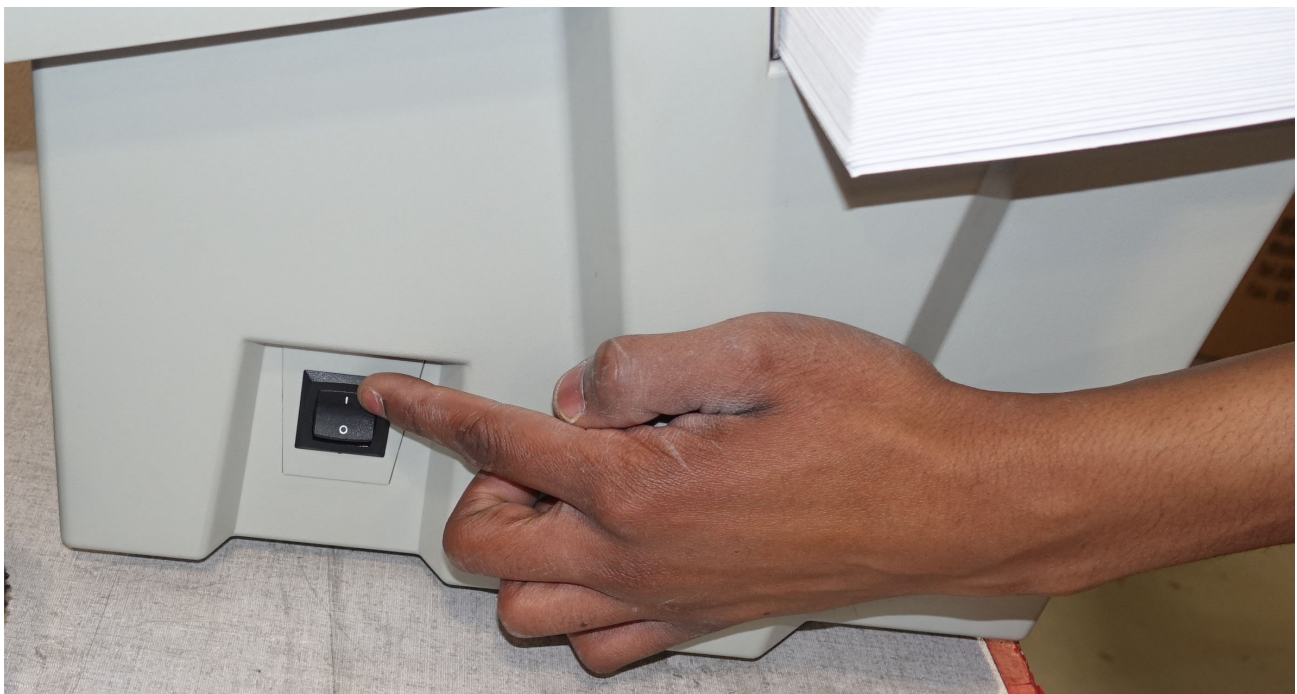
Figure 4-9: AC power switch
