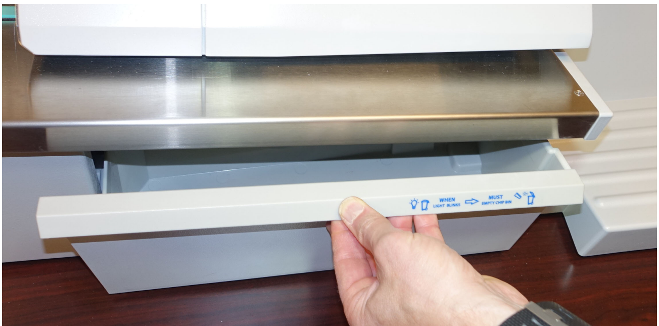
Figure 2-8: Bin tray removal interlock triggering
